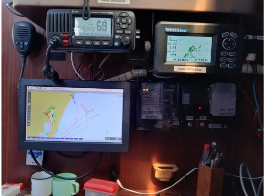
The main interest is to have sailing data screens info from KIP app, and also an AIS radar display; not really to replicate all the performances of inside equipment. In the navpod we already have 12V supply from the main switch panel (switch "navigation instruments" that also serves wind, log, speed, AIS, etc.)
