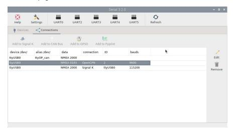
We have a ttyusb0 at the top, then a ttyusb0 at 9600 baud, which was for the handheld garmin gps when I set up openplotter 3 originally at home to test things out. Had not been able to get rid of it. It's unchecked in openCPN ever since I put the Pi on the boat.
