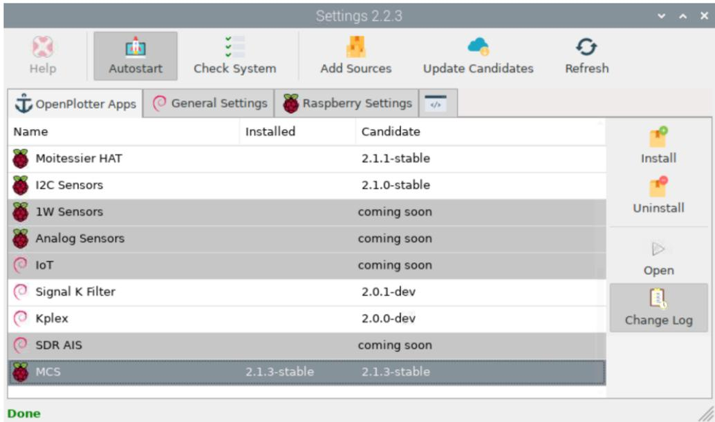
7. Install the „CAN Bus“ App for the CAN Interface on the Board. For this, select the CAN Bus App and klick install.
