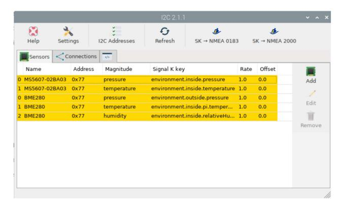
On the connection Tab, add connection to Signal K for each of the sensors:
